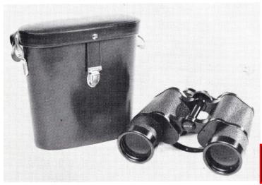
7X Magnification - 50mm Objective Diameter Exit Pupil - 7.1mm Geometrical Luminosity - 50.4 Twilight Capacity - 18.7 Field of View - 7.3 Degrees or 128m at 1,000m Apparent Field - 51 Degrees Exclusive T3M Multi - Coating Weight - 35.6 Ounces Focusing - M Models - Central E Models - Individual
