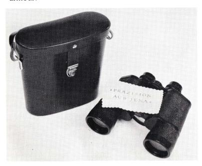
10X Magnification - 50mm Objective Diameter Exit Pupil - 5mm Geometrical Luminosity - 25 Twilight Capacity - 22.4 Field of View - 7.3 Degrees or 128m at 1,000m Apparent Field - 73 Degrees Weight - 35.9 Ounces Focusing - M Models - Central E Models - Individual Exterior Finish - Pebble Grain or Partially Rubber Armored (Individual Focus Model Only)
