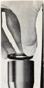
1. Remove only the protective end ring from objective barrel of 4x scope.
