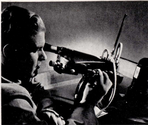
In petroleum, food, and other industries, optical methods of refractometry are used to determine concentration, density, purity.
