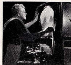
Dimensional tolerances in ten-thousandths of an inch are measured with this precise optical means.
