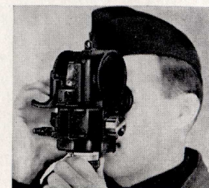
Celestial navigation keeps trans-ocean flights on course, using this Bausch & Lomb bubble sextant.
