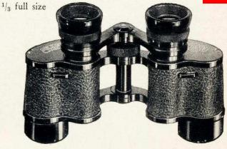
TELEXEM Magnification 6× Same as above, but with central focusing mechanism.
