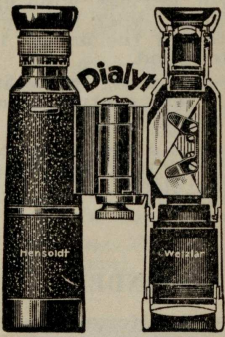
Construction of a Hensoldt telescope — showing the passage of the light through the lenses and prisms.
